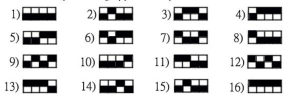
According to the above patters described, 16 transmitters (16 groups) can be set up for one-transmitter-to-many-receivers and many-transmitters-to-many-receivers connections at the same time. One transmitter unit is allowed for connecting 256 RX units in a group (4 layers).
